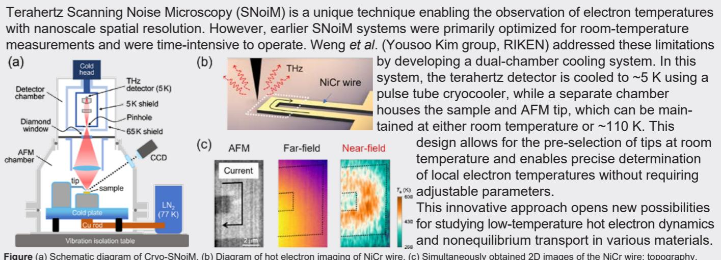
Figure (a) Schematic diagram of Cryo-SNoIM. (b) Diagram of hot electron imaging of NiCr wire. (c) Simultaneously obtained 2D images of the NiCr wire: topography, far-field and near-field (SNoIM) signals.
